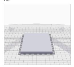
The Raised Part feature prints the part above a thin layer of supports. Turn on for the most consistent surface resistance.
